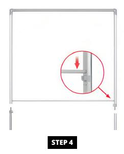
Slide the middle support bar into the frame connector pieces.
