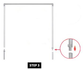
Unfold the top half of the frame and connect the male and female ends of the frame to the bottom half of the frame.
