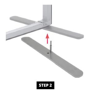
Attach the bottom half of the frame to the feet.
