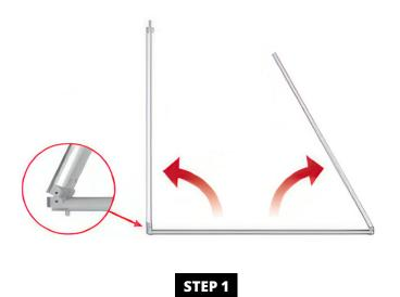
Unfold the bottom half of the frame.
